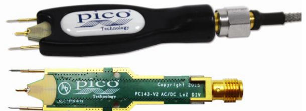
Fig. 7. Practical realisation of low cost precision passive probe.
