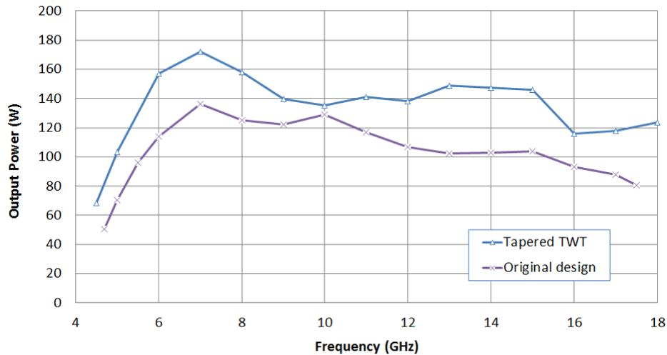
**Figure 4: Broadband performance enhancement via helix pitch profiling**
