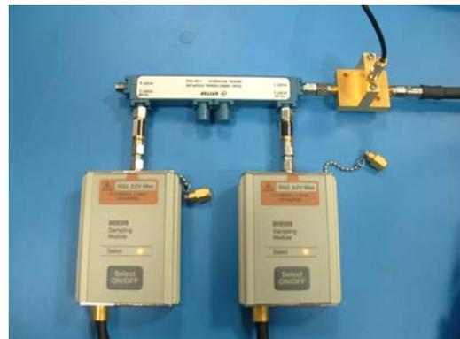
Figure 3, RF Coupler & Sampling Heads
