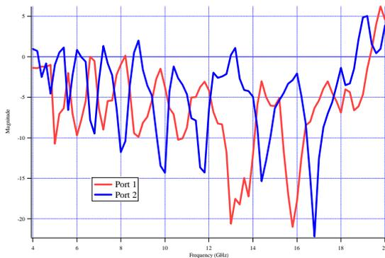
Figure 13, Antenna (anti-phase) port response
