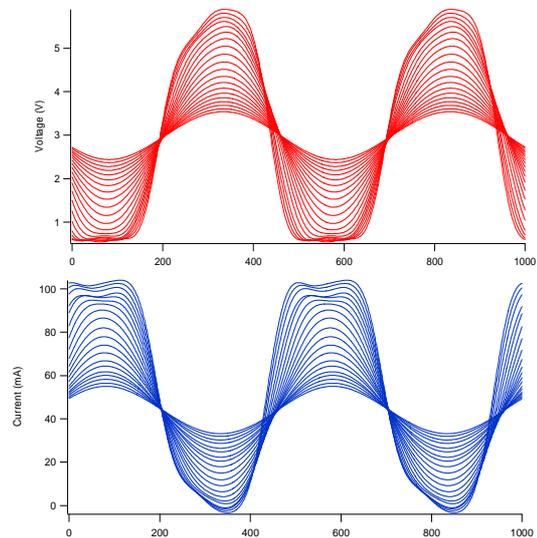
Figure 8, Output Voltage & Current Waveforms from transistor with input power
