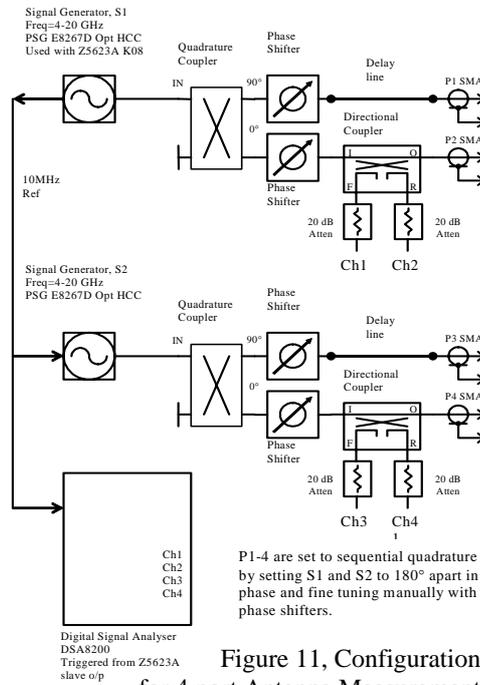
Figure 11, Configuration for 4 port Antenna Measurement
