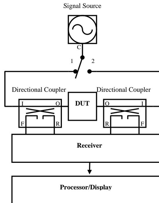
Figure 1. Basic VNA Block Diagram
