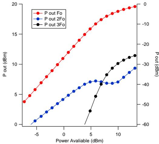
Figure 9, Fundamental, 1<sup>st</sup> & 2<sup>nd</sup> harmonic output power with increasing input power
