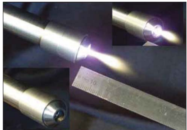
Figure 3, 2.45GHz argon plasma jet for cutting or welding applications at 3400°C.
