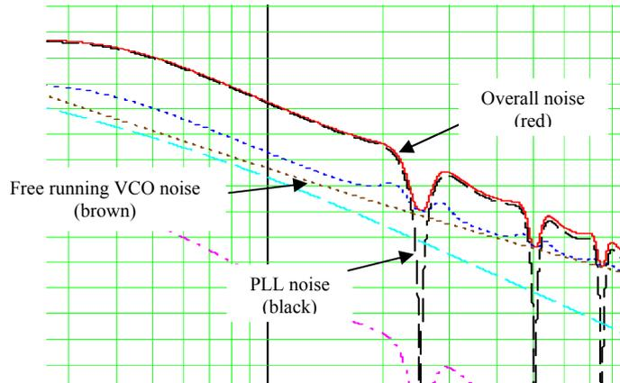
Finally a phase noise measurement on the test PLL and the free running VCO confirms that the simulation is quite a good match to the real thing (Figure 10).
