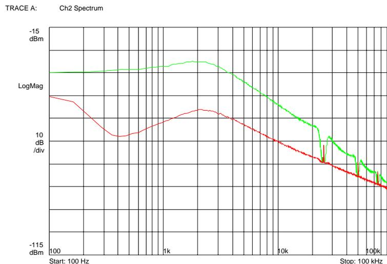
In Figure 16 the noise due to the oscillator has been increased so that it becomes comparable with the PLL noise at  $\sim 50\text{kHz}$ . The nulls at the sampling frequency and its harmonics are still present but much less evident. The noise beyond  $25\text{kHz}$  is being affected by the noise due to the VCO and by the time  $100\text{kHz}$  offset is reached the noise is dominated by the VCO. The blue trace shows the response if there were no contribution from the oscillator.
