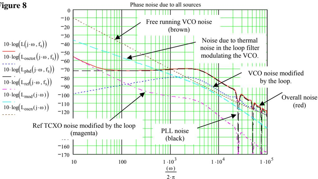
Taking a closer look at the nulls at it can be seen that the phase noise closely approaches the level of the free running VCO noise (Figure 9).
