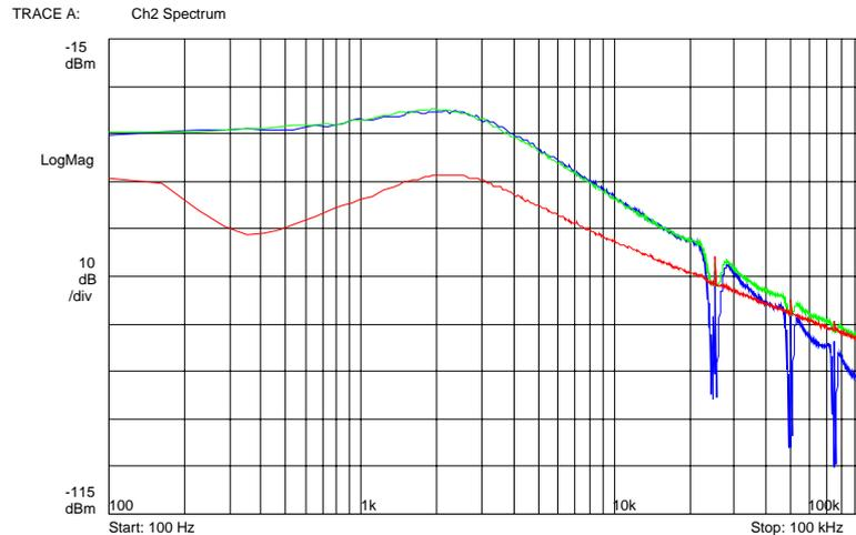
Figure 17 shows the case when the VCO noise is comparable to the PLL noise at the loop bandwidth. It can be seen that the peak at the loop bandwidth is higher due to the VCO noise and that there are still small disturbances to the noise at the sampling frequency and its harmonics even though the VCO noise is much greater than the PLL noise.
