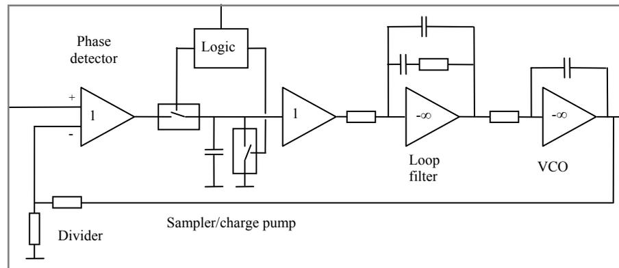
**Phase detector:** The phase detector gives us the difference in phase between two signals fed to its inputs. In the baseband circuit a differential amplifier gives us the difference between two voltages.
