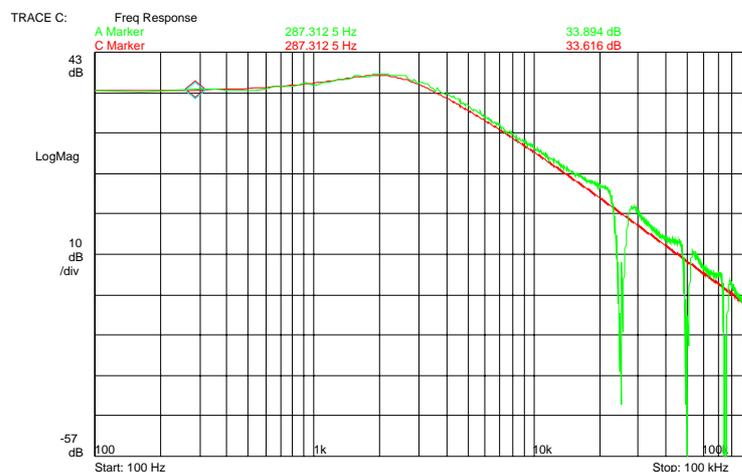
It can be seen that the sampled model has a wider bandwidth and as a result the noise due to the PLL will be higher than for the continuous time model outside the loop bandwidth except in the regions close to the sampling frequencies and its harmonics where the PLL noise is heavily suppressed.
