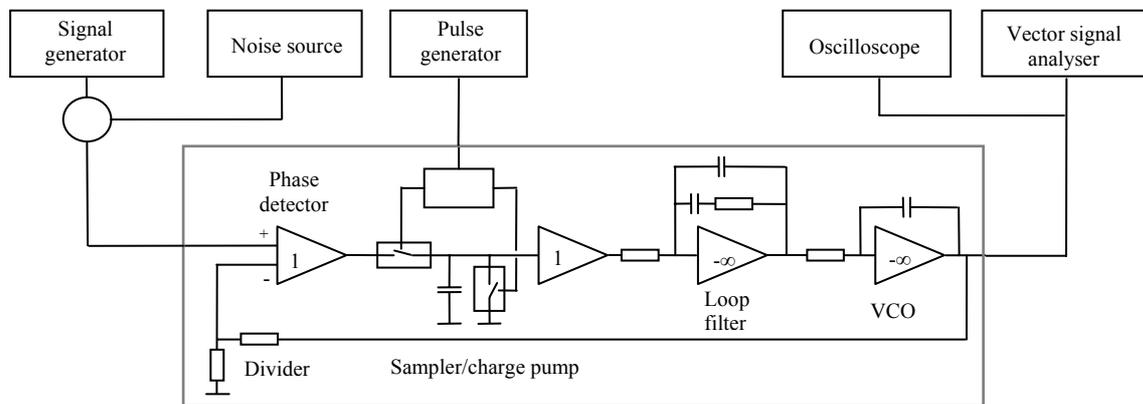
The sampler is first disabled by setting the series switch permanently on and the shunt switch off to create a continuous time model and the signal generator turned off so that the response may be measured using broadband noise as the input. The measurement is accomplished by taking many averages at the output. The more averages the smoother the trace.
