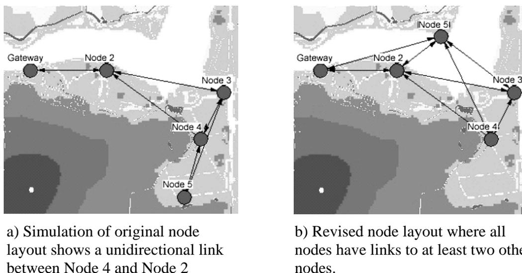
Figure 4: Results from the simulator showing possible communication links between the nodes.
