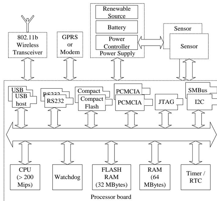
Figure 2: The schematic of a sensor node, where the grouping of components into units, indicated by the dashed outlines, denotes a sub-assembly.
