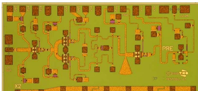
Figure 5. Photograph of the 48 GHz LO chain
