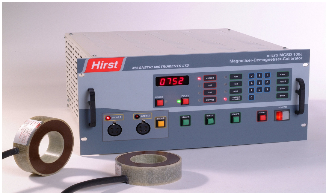
Figure 12. Illustration of a “maximal” embodiment of a dual output automatic magnetic calibration system.
