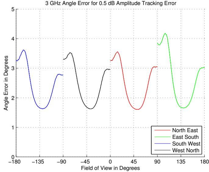
Figure 4: AOA Calculation Error for the Antennas in isolation at 3GHZ
