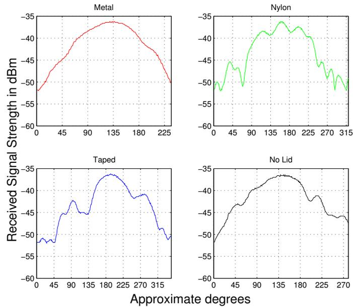
Figure 5: Amplitude measurements taken at 3 GHz with different lids
