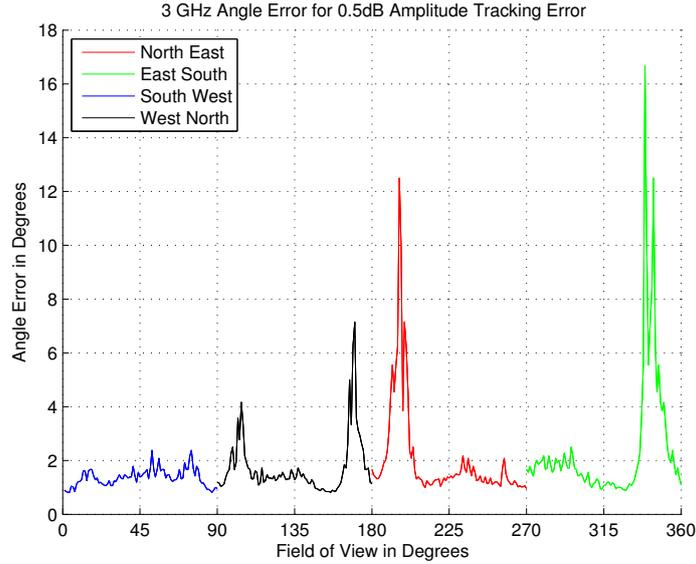
Figure 8: System Angle Error for a 0.5 dB Tracking Error at 3 GHz
