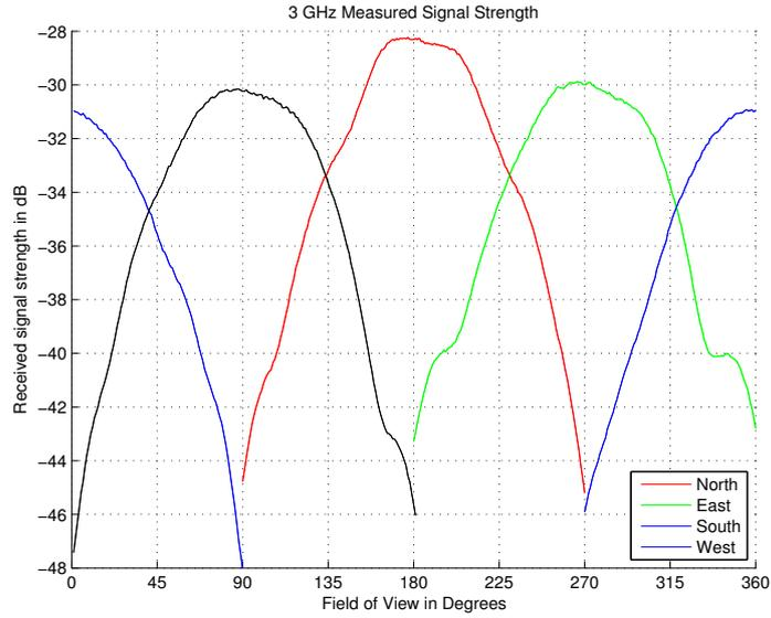
Figure 6: System Amplitude measurement at 3 GHz
