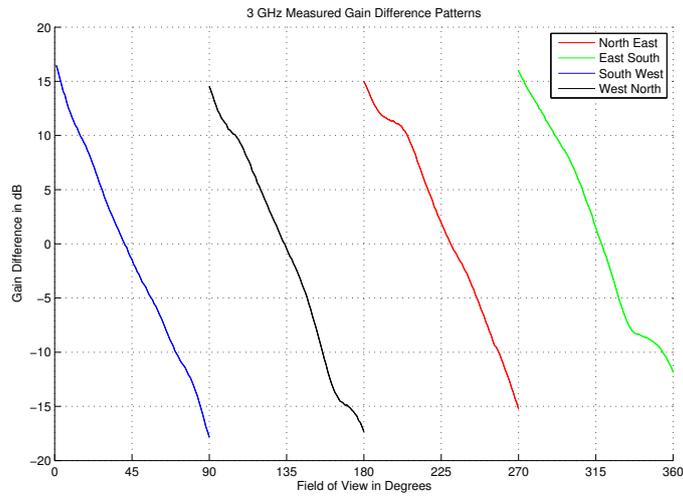
Figure 7: System Gain Difference at 3GHz
