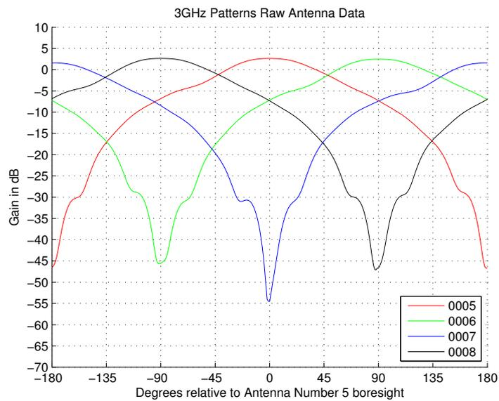
Figure 2: Antenna Gain Patterns
