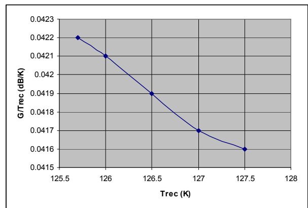
Fig. 4 G/T Ratio versus Receiver Noise Temperature (0.5 K drift)
