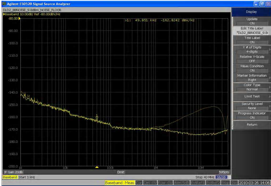
Figure 7. DLD2 BBNOISE and Noise Floor (delay line replaced with 6. in cable) , 4GHz setup
