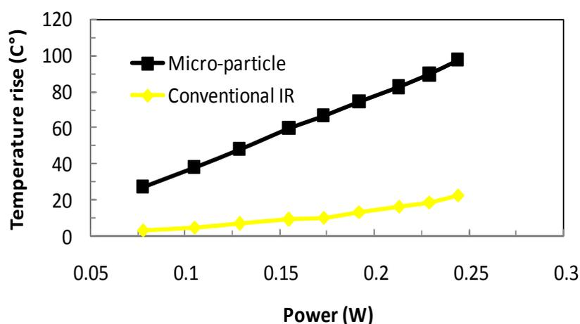
**Figure 10:** Temperatures measured on the channel region of the AlGaIn HEMT using micro-particle and conventional IR techniques.
