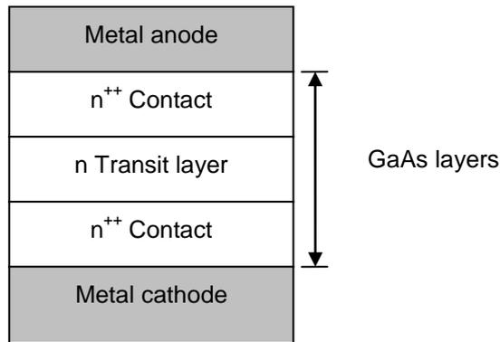
**Figure 3:** Structure of the GaAs Gunn diode.
