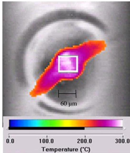
**Figure 5:** Typical IR temperature image measured on the coated top contact of the electrically powered GaAs Gunn diode.  $\times 5$  magnification. Power = 6 W,  $T_{\text{ambient}} = 80\text{ }^{\circ}\text{C}$ .
