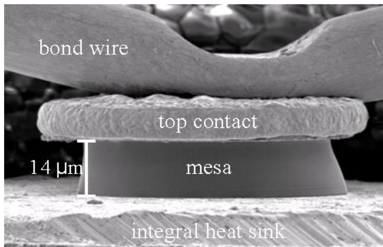
**Figure 4:** SEM image showing the construction of the Gunn diode.
