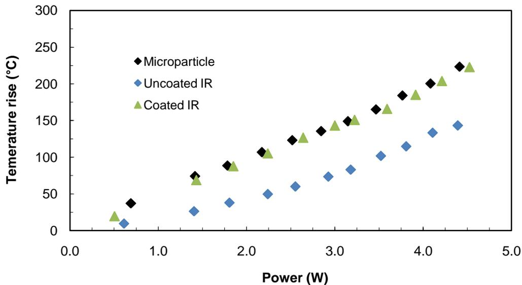
**Figure 7:** Comparison showing the peak temperature rise measured on the metal top contact of the Gunn diode using the micro-particle and conventional IR techniques.
