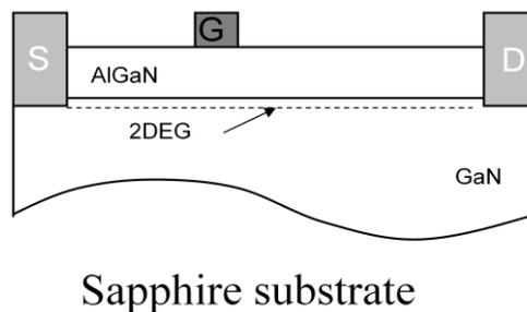
**Figure 8:** Construction of the AlGaN/GaN HEMT.
