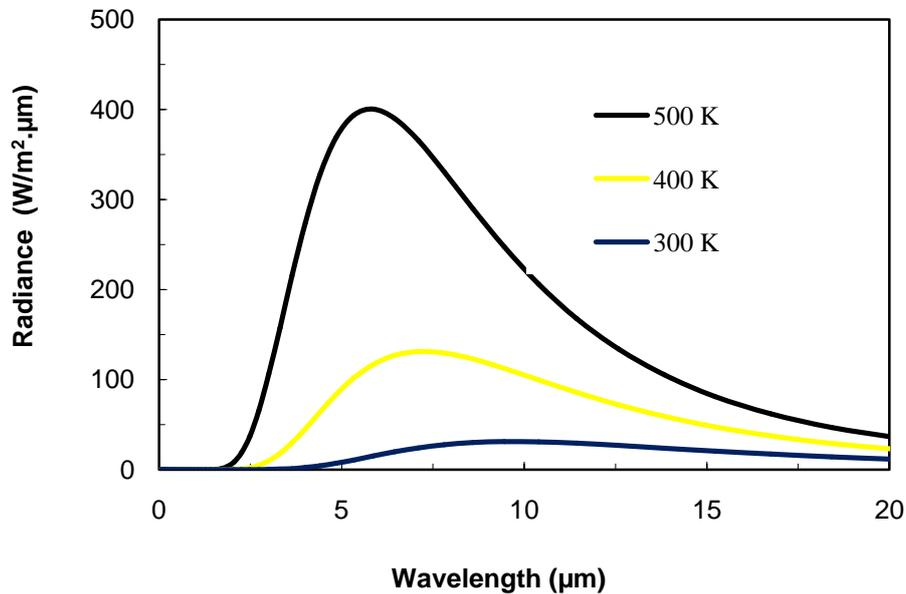
**Figure 1:** Spectral distribution of emitted IR radiation from an ideal black body source.
