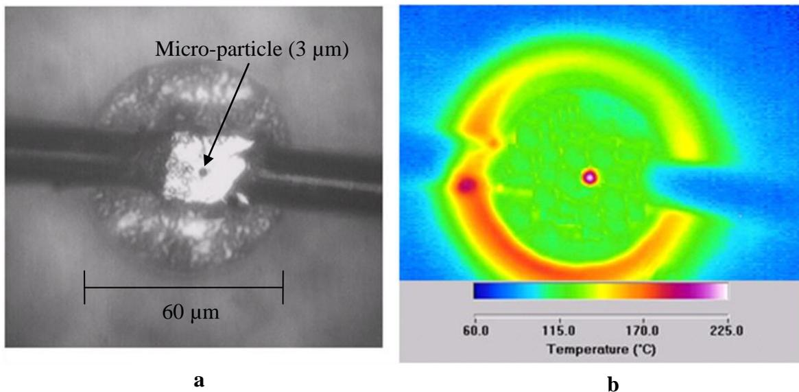
**Figure 6: a)** Optical image ( $\times 20$  magnification) showing a carbon micro-particle ( $3\text{ }\mu\text{m}$  diameter) deposited on the gold top contact of the Gunn diode. **b)** IR temperature image of the micro-particle on the device (Power level = 4 W).
