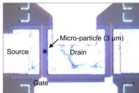
**Figure 9:** Optical image showing the micro-particle IR sensor (3  $\mu\text{m}$  diameter) placed in the channel region of the AlGaN HEMT.
