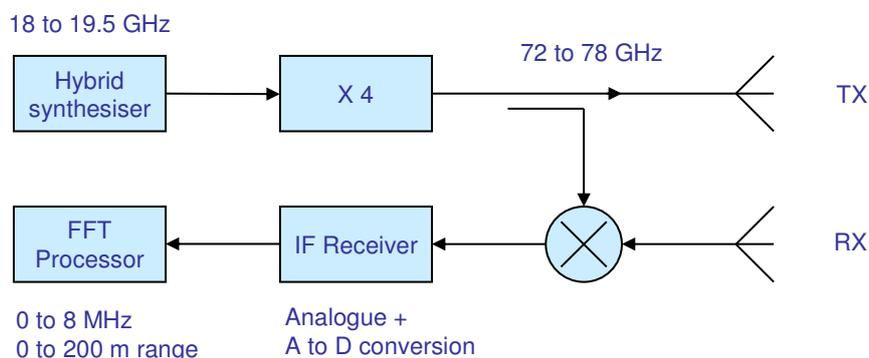
Figure 12 mmWave Radar System
