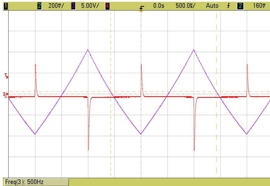
Figure 11 VCO Control Voltage and Loop Error Voltage
