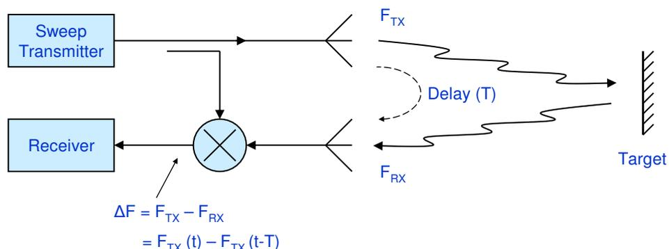
Figure 1 FMCW RADAR Architecture
