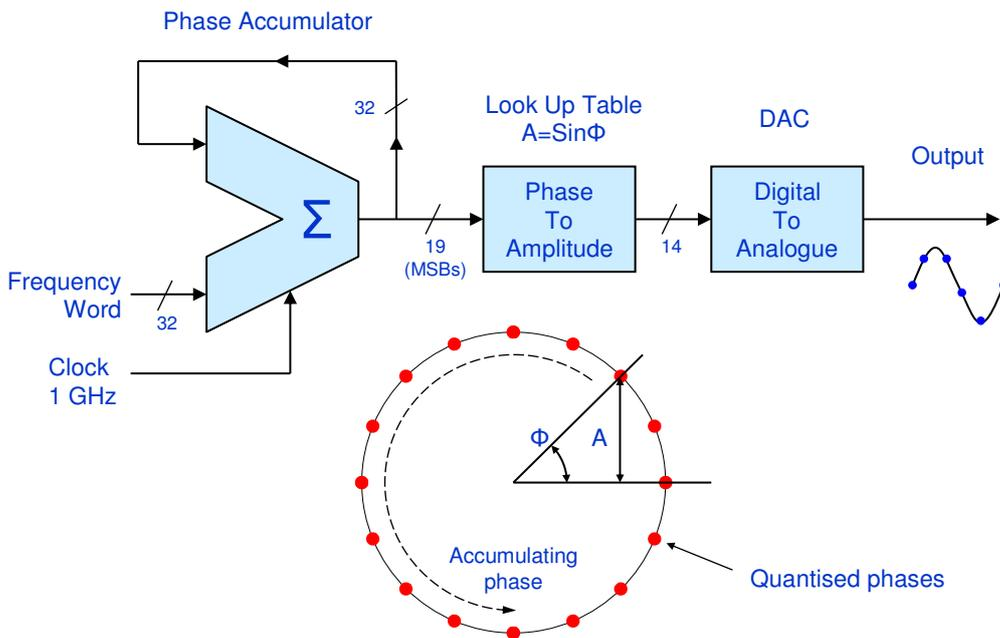
Figure 5 DDS Synthesiser Core
