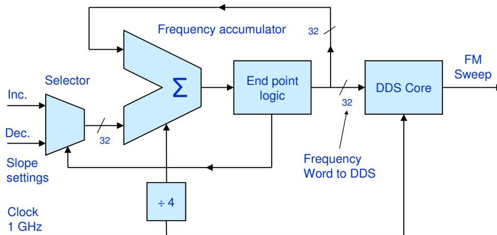
Figure 7 DDS With Frequency Ramp
