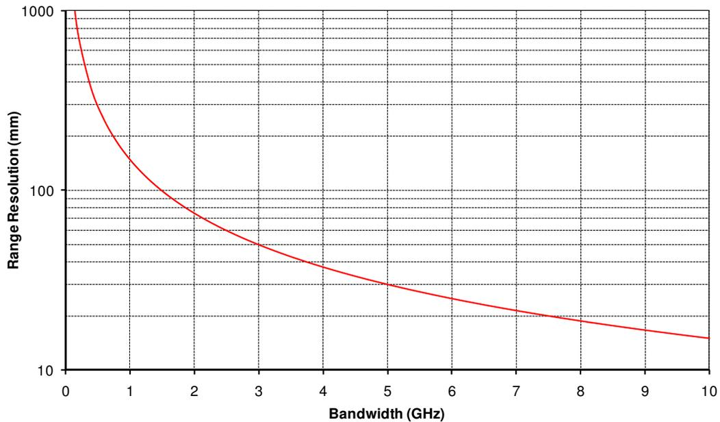
Figure 3 Resolution versus Bandwidth
