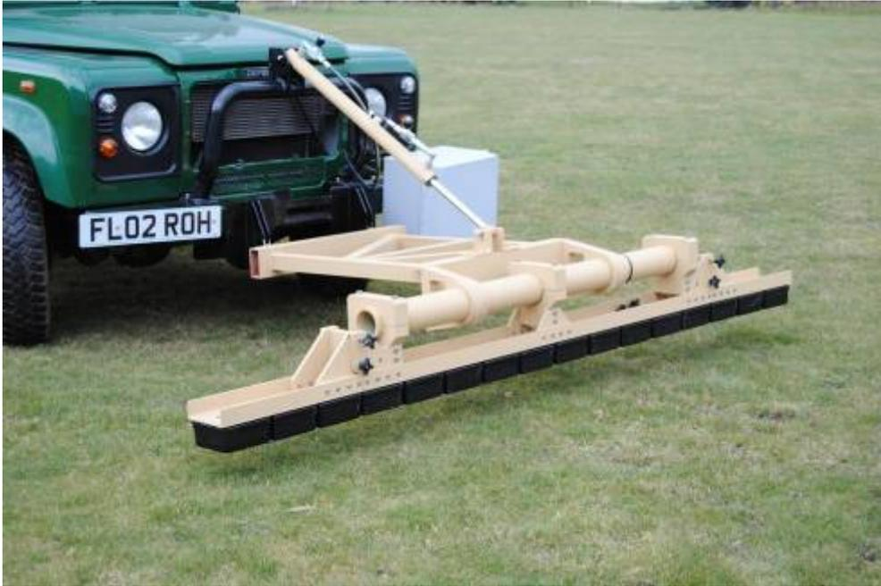
Figure 6 COBHAM 16 channel radar system
