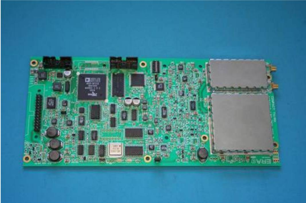
Figure 5 Radar transmitter receiver and processor
