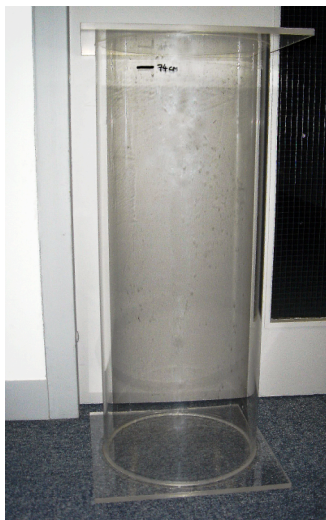
Figure 1: A body phantom is used to test in-body antenna performance
