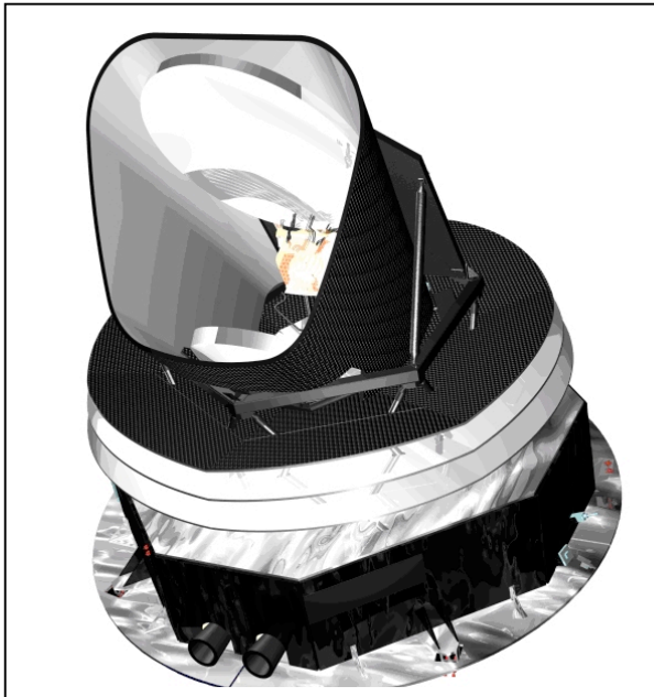
Figure 1-1 Planck Telescope Showing SVM, Off-axis Antenna, LFI and HFI Modules
