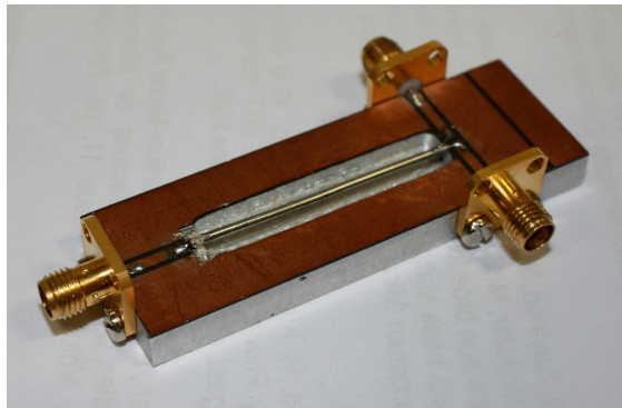
Fig. 3: Simple coaxial cable transmission line balun.
