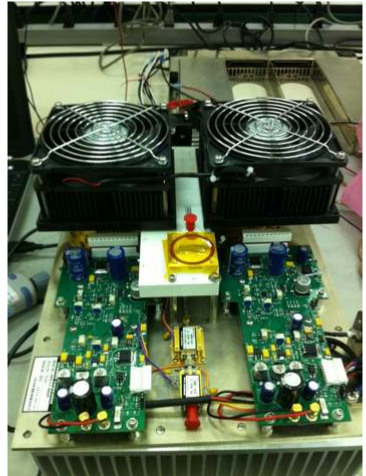
Complete Pulsed 1 kW X-Band Radar PA Demonstrator
