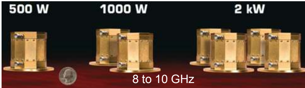
Examples of Radially Combined PA's using Cree GaN MMICs
